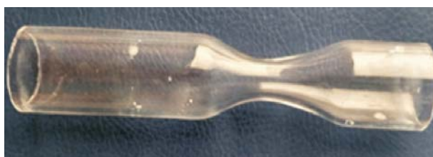
Fig. 1. High-Q cylindrical resonator SSG made of industrial quartz tube
